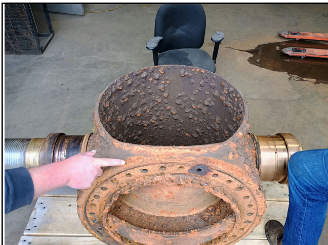
Valve fully disassembled at Mar-Tech facility to identify areas of wear and feasibility to repair.
